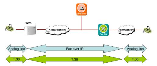
Figure 1 - Typical network for VoIP running Fax (T.38)
